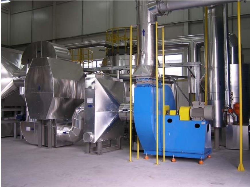
Picture 1: Installation for mineralization of MSW (10t/24h)
